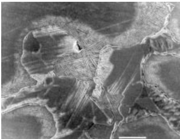
Figure 11 Scanning electron micrograph of a polished and etched, axially-sectioned, as-cast Spartan Plus specimen after fracture, showing crystallographic features in the palladium solid solution suggestive of twinning. A lamellar eutectic constituent in the interdendritic region is evident at higher magnification. Bar = 100 \mu\text{m} .
